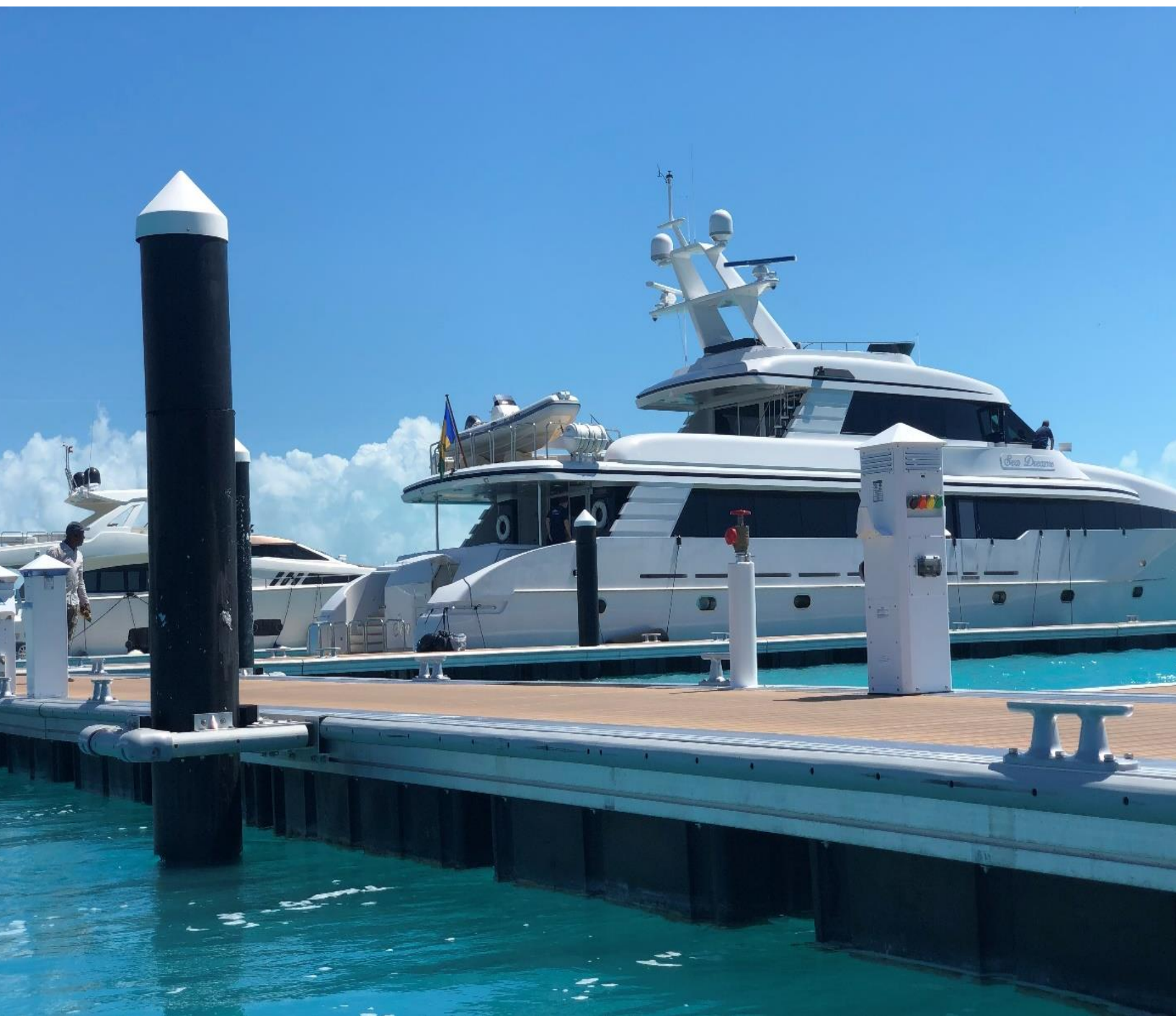
Marina Technologies System D-260 aluminum-framed dock system designed for mega-yachts.
