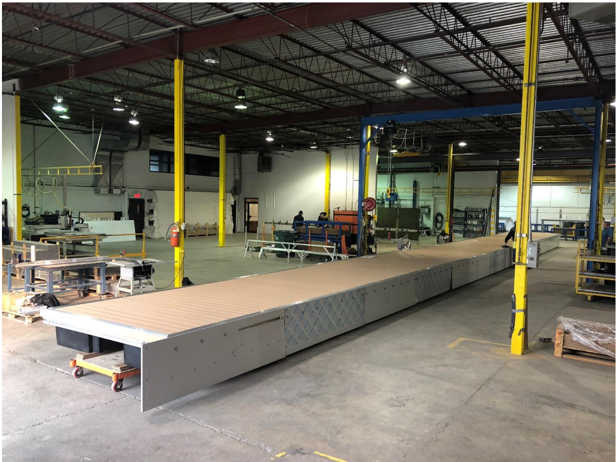
MTI's Floating Oil Containment System under fabrication.
